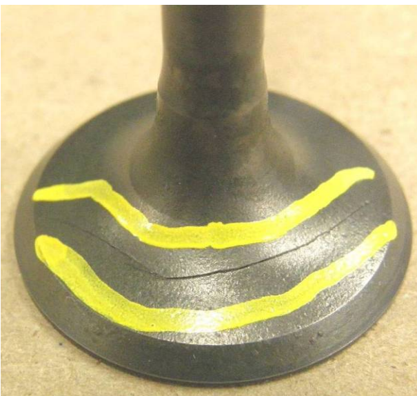
Figure 26: Cracked Valves from E15 Verado 1B812776, Bottom Valve in Cyl. 3 Left, and Top Valve in Cyl. 6 Right
