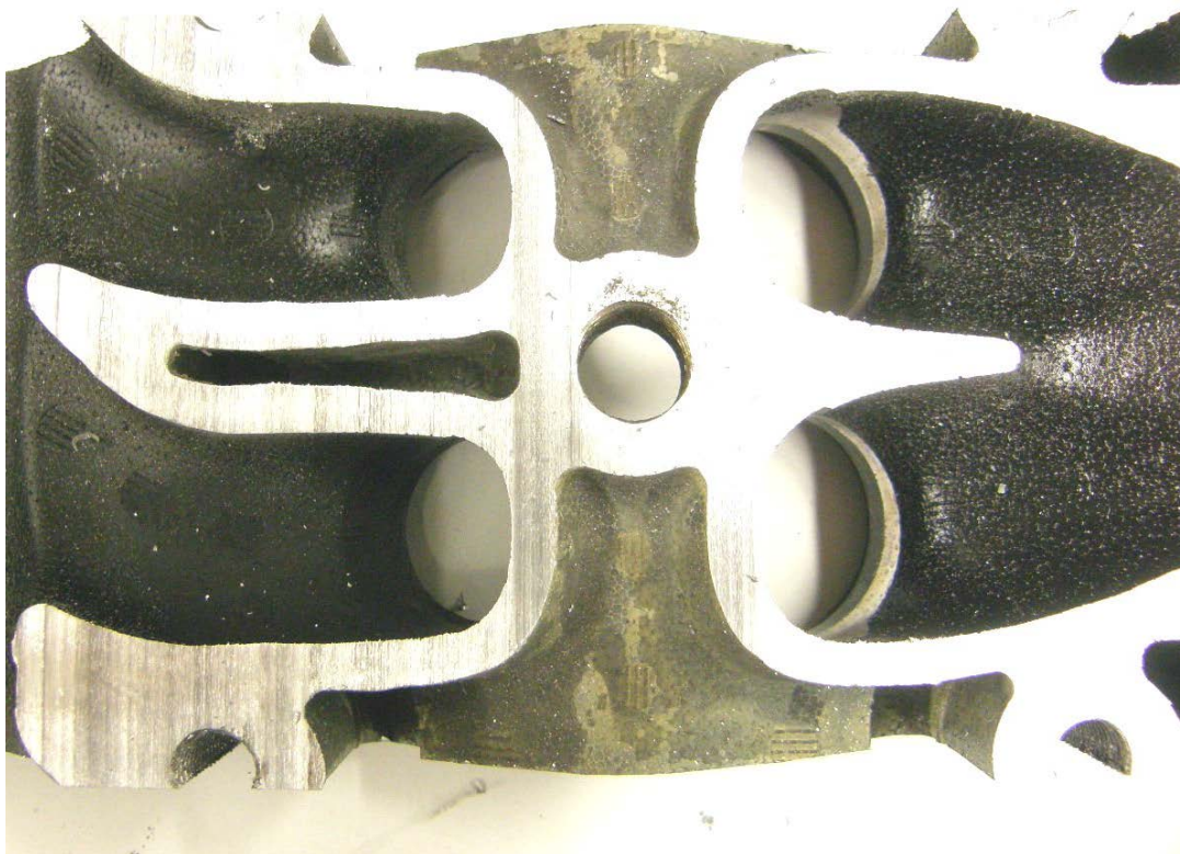
Figure 31: Photo of Section of Cylinder 3, E0 Verado 1B812775A, Exhaust Ports on Left
