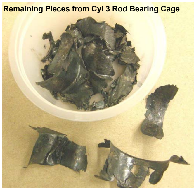
Figure 44: 200HP EFI Bearing Failure Pictures
